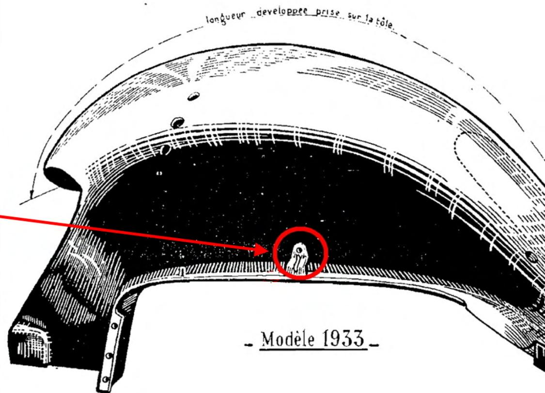
R 119 - Protection embout barre repose capot
